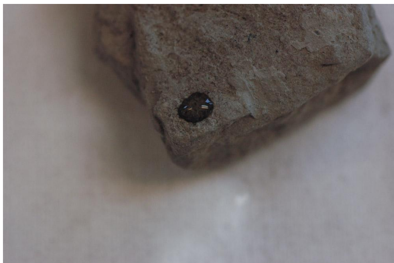
Figure 2. T-4 sample after light rinsing with de-ionized water. The HCL drop produced no bubbles.
